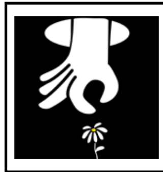
1 Protected against access to dangerous parts by hand pressure. Protected against solid foreign bodies Ø50mm.
