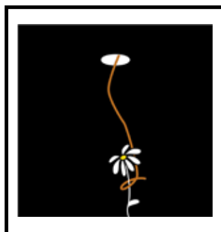
4 Protected against access to dangerous parts by a wire. Protected against solid foreign bodies Ø1mm.
