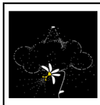
5 Protected against access to dangerous parts by a wire. Protected against dust.
