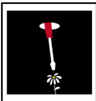
3 Protected against access to dangerous parts by a tool. Protected solid foreign bodies Ø2.5mm.
