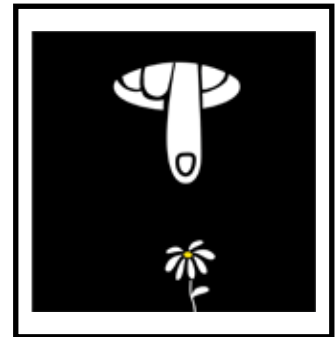
2 Protected against access to dangerous parts by fingers. Protected against solid foreign bodies Ø12.5mm.
